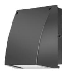
37, 57 and 62 Watt SLIM Wall packs are designed to cover the footprint of most traditional wall packs. They are suitable for mounting heights from 20' to 30', and replace HID Wattages from 200W MH to 320W MH. These ultra-high efficiency fixtures are available in cutoff or full cutoff models.
